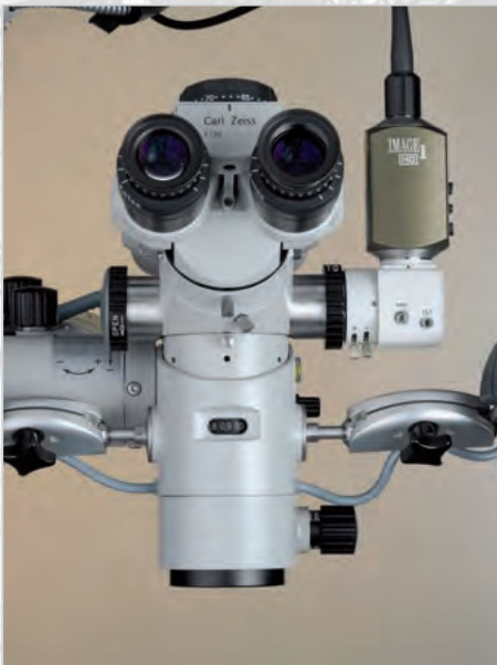
Direct adaption to the VARIO operating microscope from Carl Zeiss Meditec
