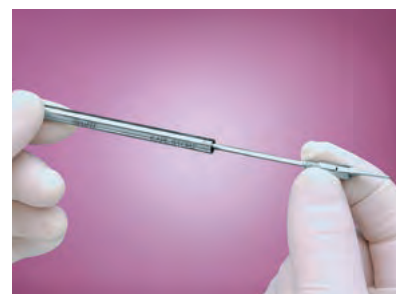
In the case of instruments with three parts, you then release the bayonet mount by turning it 90° and pulling the working insert out of the sheath. Done!
