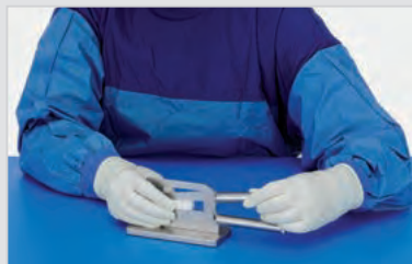
Fig. 2: ... and fixated with the "holding-down clamp" handle.
